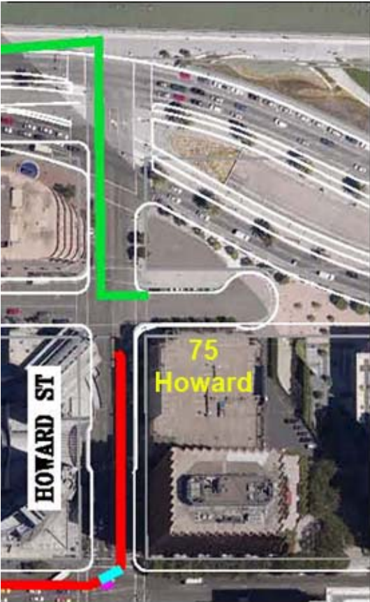
2 high pressure sewer mains (SF PUC map)
